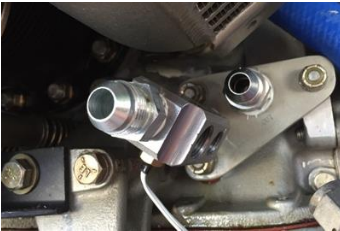
Engine temp sensor shown mounted in oil cooler fitting block
